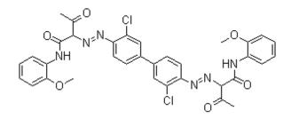
**FASTNESS PROPERTIES** Acid 5 ISO 787-4 Alkali ISO 787-4 5 Water 5 ISO 2836 **Ethanol** 5 ISO 2836 **Xylene** 4 ISO 2836 **MEK** 3 ISO 2836 DOP 5 ISO 2836 Heat / 150°C, 10 min ISO 787-21 Heat/ 210°C, 10 min 3 ISO 787-21 Light 1/3 SD 5 ISO 105-B01 Light 1/25 SD 3 ISO 105-B01
